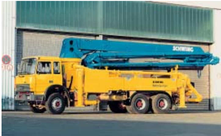
Schwing concrete pump.
