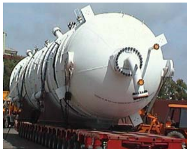
Pressure vessel out of SA 387-22-2 1
