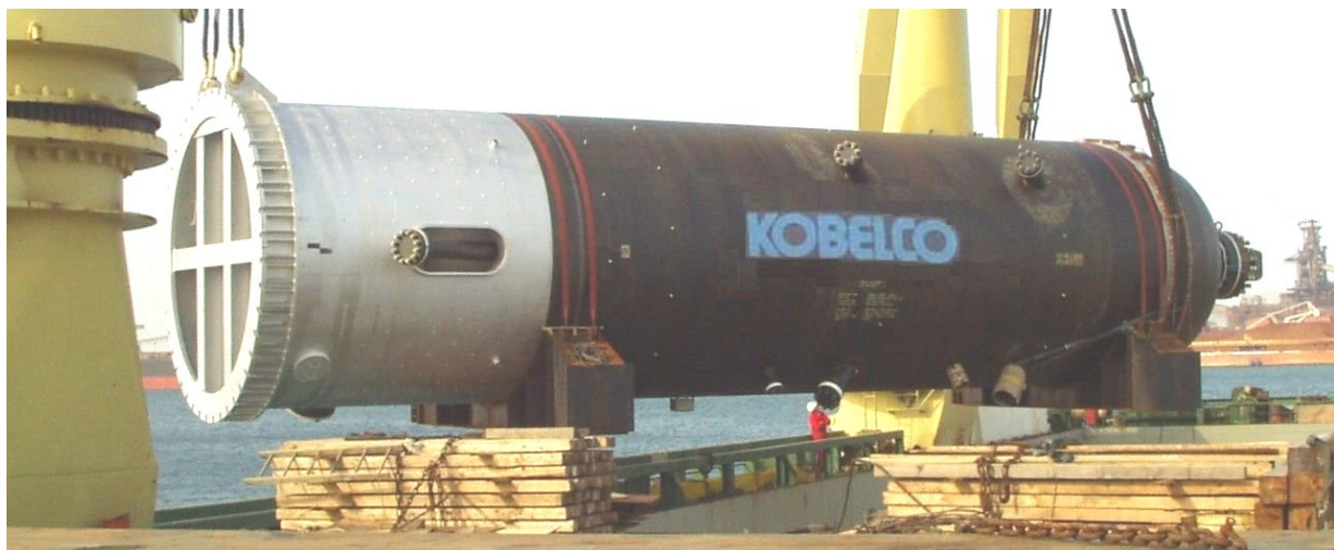
585 t pressure vessel out of SA 542-D-4A for a refinery project 2
