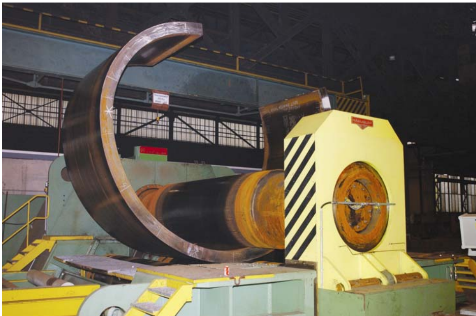
Cold bending of a 240 mm thick shell section in the Heavy Fabrication Division shop.
