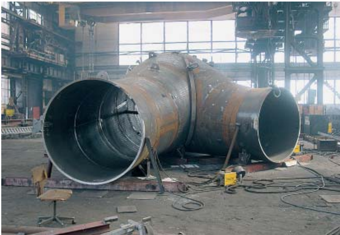
Figure 6: Pipes made of DILLIMAX 690 for the penstock linings of the hydropower plant Kárahnjúkar (Illustration used with the kind permission of DSD Noell GmbH, Würzburg, Germany)
