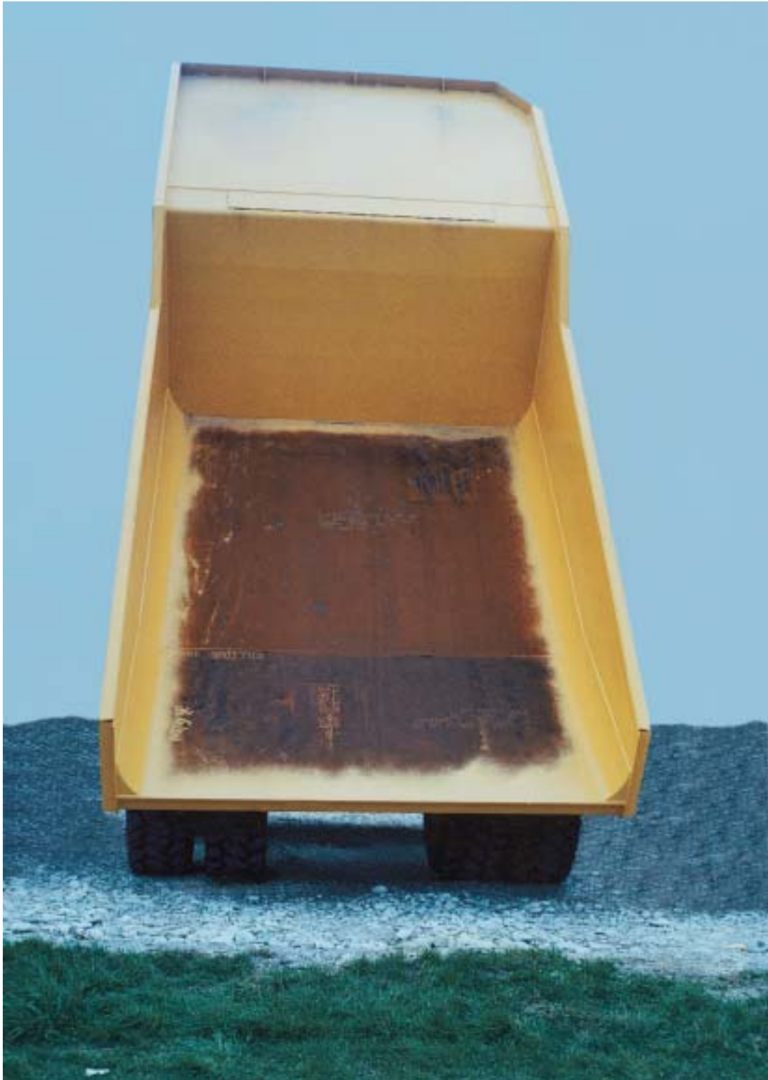
Figure 21: Welded truck dumping body made of DILLIDUR 400 V, plate thickness 10 mm
