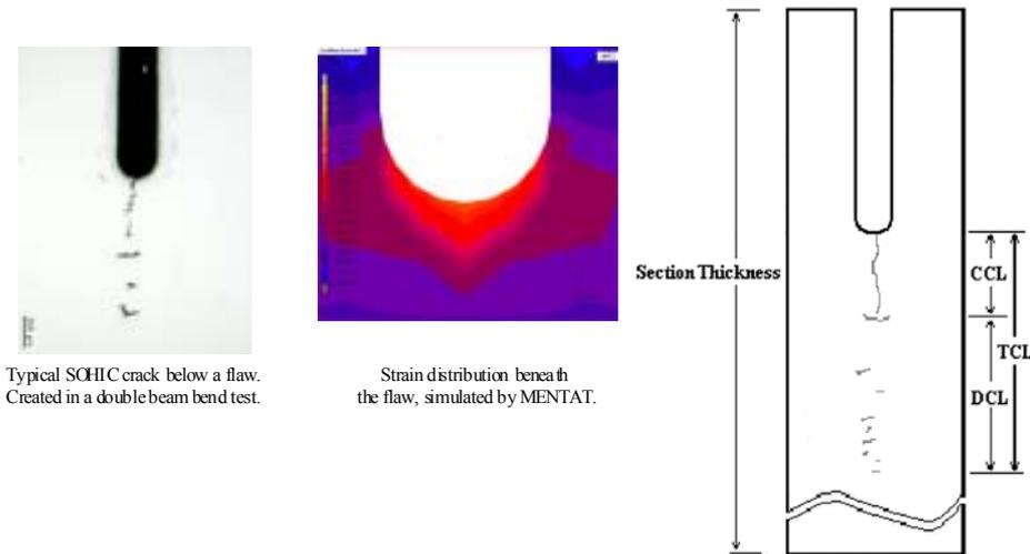
*Figure 4: SOHIC type cracks in the area of a stressed notch, strain distribution at the bottom of a notch and evaluation criteria for SOHIC cracking.*
