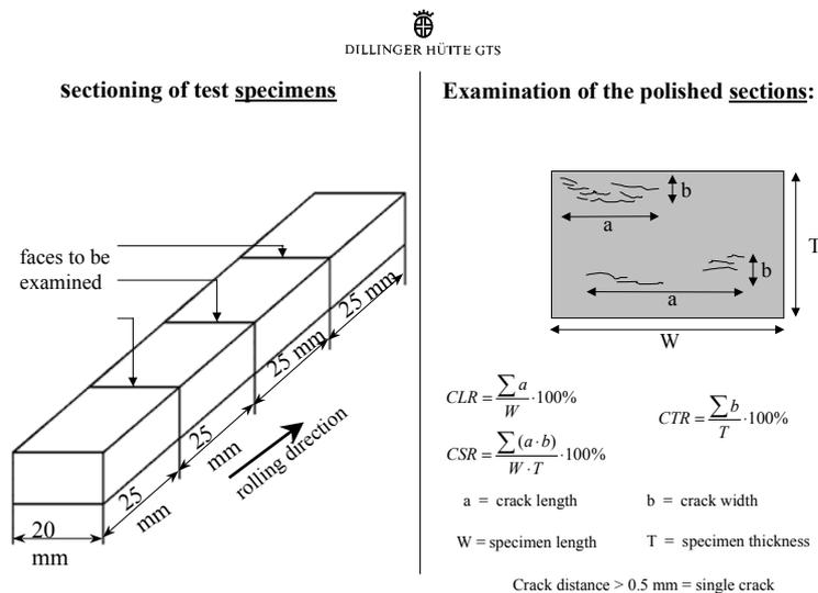
Figure 2: HIC test evaluation according to NACE TM 0284
