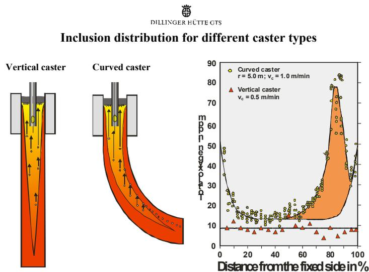
Figure 7: Differences between different continuous casting types
