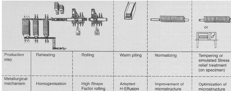
Figure 8: Production steps in the plate mill
