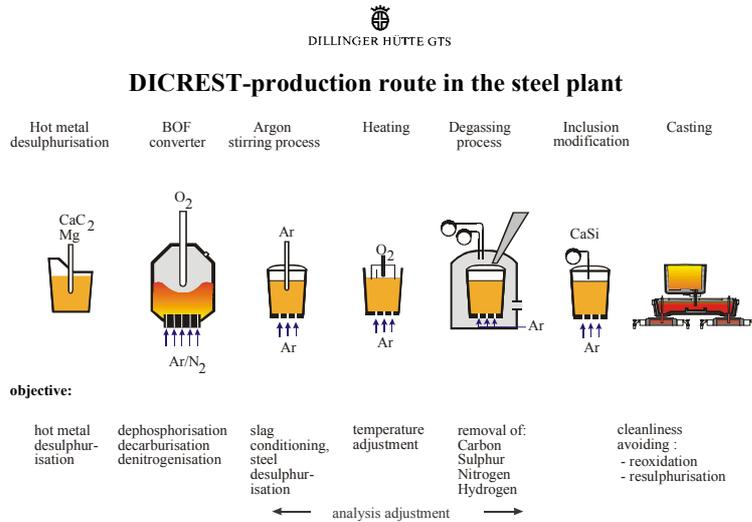
Figure 5: Production route in the steel plant
