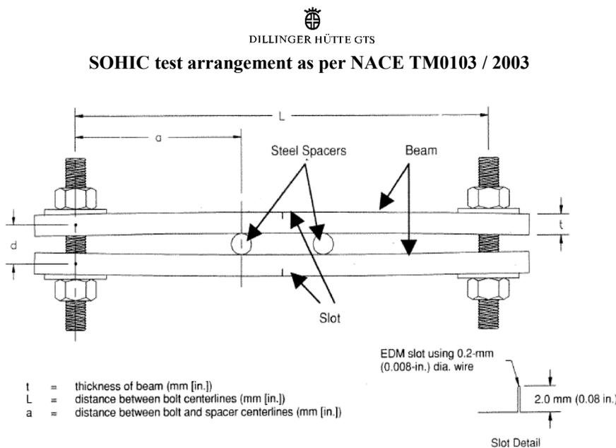
NACE TM0103 – Full Size Double-Beam Test Specimen Design
