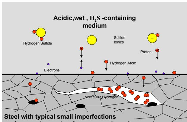
*Figure 1: Sour service damage mechanism*
