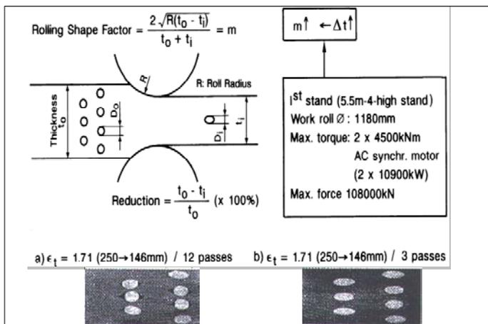
Figure 9: Influence of high shape factor rolling on plate core deformation
